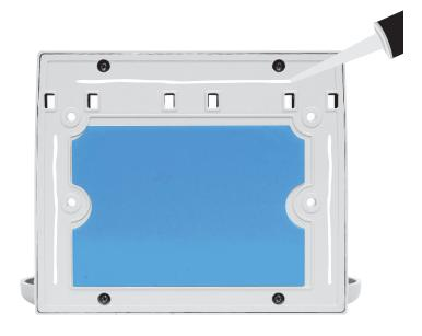
Before removing the blue tape, use adhesive caulk and lay a small bead around the outside of the back plate as shown in the graphics above
