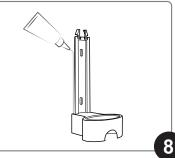
Apply a bead of bathroom-grade silicone around the edge of each bracket unit.
