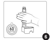
Press entire bracket against desired surface for 60 seconds to ensure bracket has adhered to surface.
