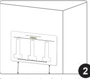
Place the template on the wall, make sure it is level. Template should be placed 48 inches from floor to bottom of template. **Tub:** Dispenser(s) should be centered directly
