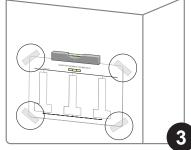
Put level to top of template and tape corners of template in desired spot. Do not use glue on the template.
